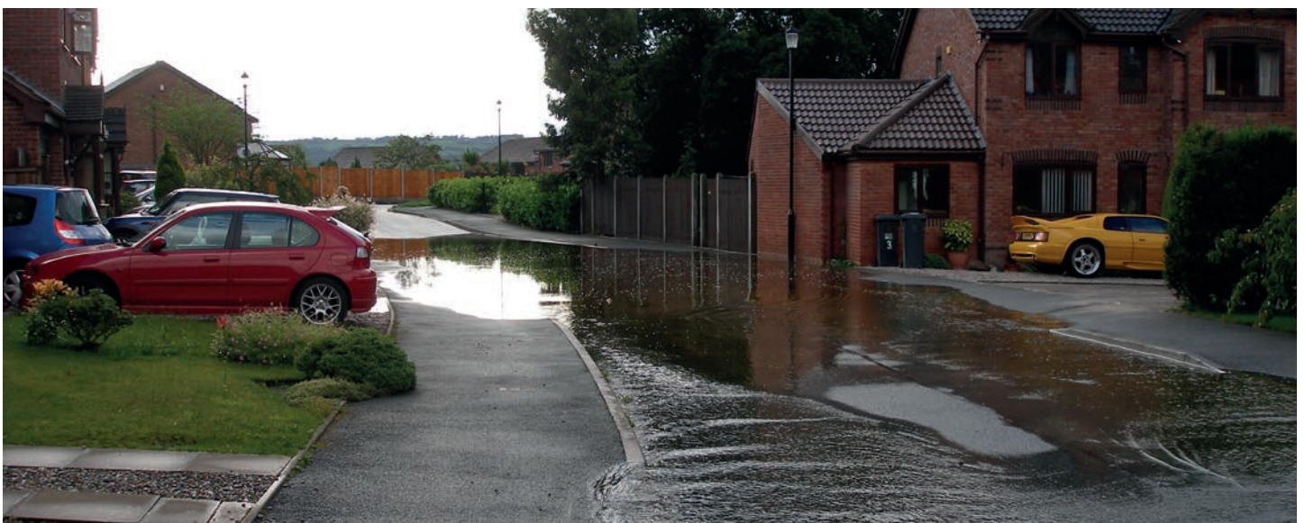
Surface water run off at the back of the Thames Drive estate, with water flowing off the hills onto Plover Drive in this example
