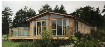
Typical Monopitch Timber (Vertical & Horizontal) Clad Lodge. Pale Grey Powder Coated Aluminium Frames. Galvanised Rainwater Goods. Pressed Metal roof. Timber Skirt and Deck Posts
